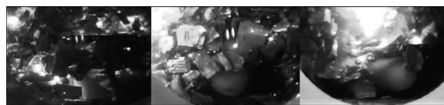
Figure 3. Real-time images of electrostatic discharge (arcing) between stirred Mg turnings in THF in a high field density microwave reactor (Monowave 300). Clearly visible is the stir bar at the bottom of the vial.
